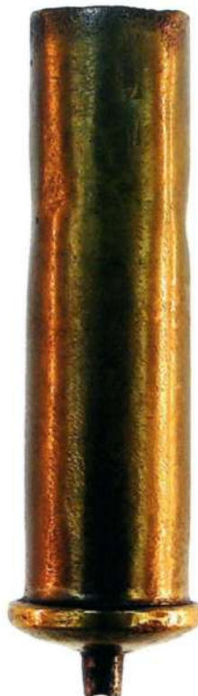
Fig. 22b: Lenoir brass case with steel nipple. Overall length: 64.1 mm; diameter base: 18.1 mm. Antonius Rauch collection.
