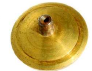
Fig. 21a: Base view of the rosette with its steel nipple.
