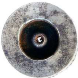
Fig. 42: 16 Gauge Morse shotshell, solid steel base with integral nipple, type II Two-piece case; a drawn brass tube is soldered onto a turned solid steel base with an integral nipple; the steel base forms a rim; it comes without rubber washer and cap. Case length: 55.9 mm; rim diameter: 20.8mm. Ex Berkeley R. Lewis collection.
