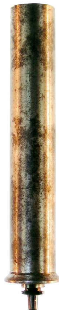
Fig. 26: So-called 16.26 mm (.64) "Picherau" steel case. Total length: 120 mm. Antonius Rauch collection.
