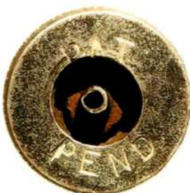
Fig. 43: 12 Gauge (Morse-type?) shotshell "PAT PEND" Two-piece case: drawn brass tube fixed on a turned steel base which has a screwed-in steel percussion nipple with hexagonal base; impressed "PAT PEND" head stamp (means "patent pending"); the rim of the steel base is crudely knurled. Overall length: 72.7 mm; rim diameter: 22 mm; length of steel insert: 8.2 mm.
