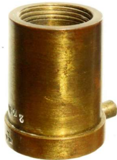
Fig. 31c: The case mouth is threaded to secure the round ball.
