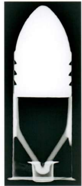
Fig. 38: .69 Morse, brass case, type I a One-piece construction; drawn brass case flared at base to rim; rubberized fabric washer and copper cap; smooth pointed lead bullet; form of anvil is the single brass wire “hairpin” type (type I a), see X-ray. Case length: 39.2 mm; overall length 53.8 mm; bullet diameter: .676 inch; exterior case mouth diameter: .720 inch; rim diameter: 21.7 mm.
