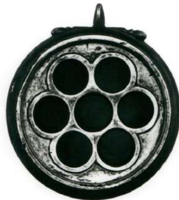
The muzzle of the gun with the bundle of its seven smooth bore barrels of .30 inch caliber.
