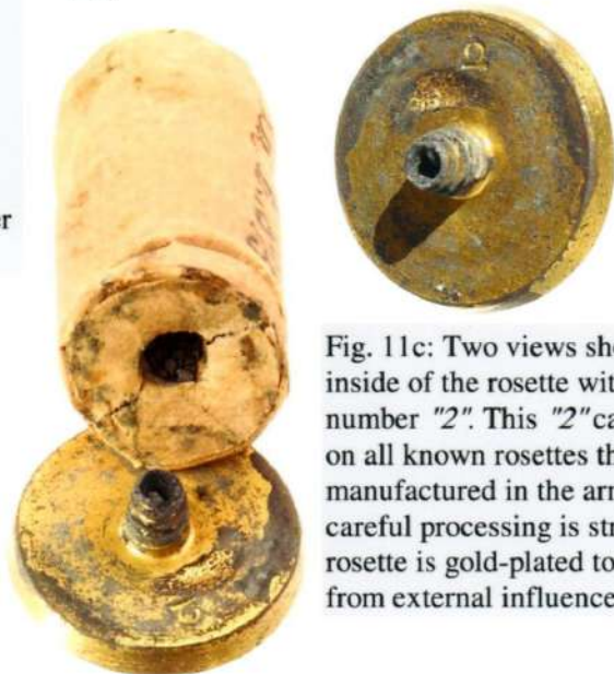
Fig. 11b: The view of the base of the turned rosette with a recess for the ignition compound and screwed-in iron disc with ignition orifice. Iron used as a more resistant metal to impact than brass. Diameter of the rosette: 22.55 mm.
