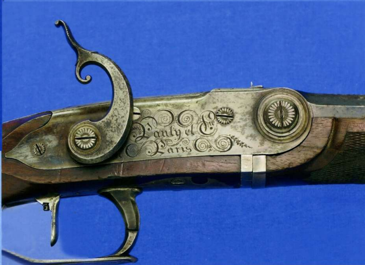
The open end of the barrel tilting up at breech and with recess for the rosette. The hole on top of the frame is a device for discharging excess gas pressure.
