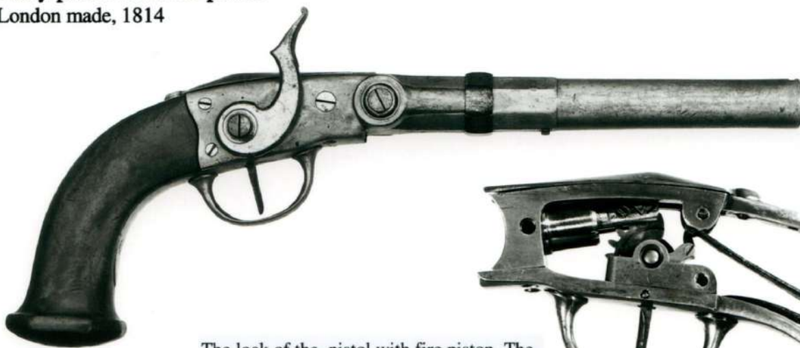
The lock of the pistol with fire piston. The air tight piston is driven by a cog-wheel.
