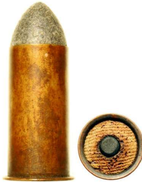
Fig. 38: .69 Morse, brass case, type I a One-piece construction; drawn brass case flared at base to rim; rubberized fabric washer and copper cap; smooth pointed lead bullet; form of anvil is the single brass wire “hairpin” type (type I a), see X-ray. Case length: 39.2 mm; overall length 53.8 mm; bullet diameter: .676 inch; exterior case mouth diameter: .720 inch; rim diameter: 21.7 mm.
