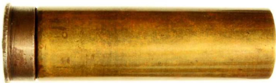
Fig. 43: 12 Gauge (Morse-type?) shotshell "PAT PEND" Two-piece case: drawn brass tube fixed on a turned steel base which has a screwed-in steel percussion nipple with hexagonal base; impressed "PAT PEND" head stamp (means "patent pending"); the rim of the steel base is crudely knurled. Overall length: 72.7 mm; rim diameter: 22 mm; length of steel insert: 8.2 mm.
