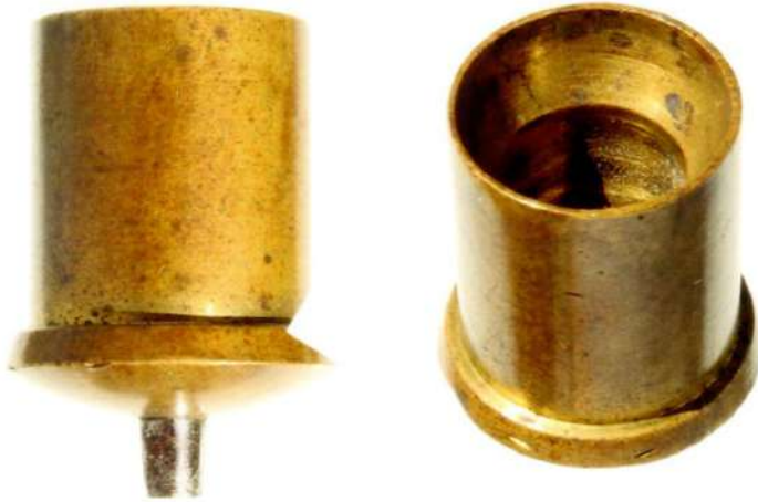
Fig. 20: A very heavy thick-walled two-piece brass case with an inserted steel nipple acting as the anvil, according to the 1823 patent by Henri Roux. The case mouth is chamfered to accept the round ball. The caliber of the turned case is 16.25 mm. Overall length: 29.9 mm; diameter case: 17.9 mm; diameter rim: 21.0 mm. This is the cartridge which I had formerly erroneously called "Pauly Type III" (see Preface).
