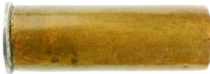
Fig. 42: 16 Gauge Morse shotshell, solid steel base with integral nipple, type II Two-piece case; a drawn brass tube is soldered onto a turned solid steel base with an integral nipple; the steel base forms a rim; it comes without rubber washer and cap. Case length: 55.9 mm; rim diameter: 20.8mm. Ex Berkeley R. Lewis collection.
