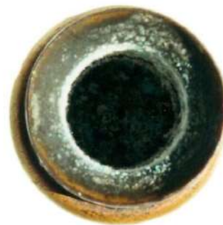
Fig. 15b: A look into the extremely thick-walled cast case. All known cases of this type are made with thick walls. Case wall thickness: 3.4 mm.
