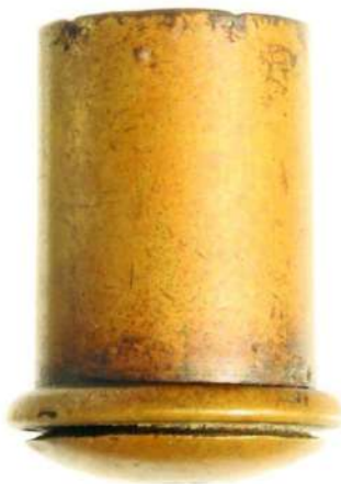
Fig. 15a: 15 mm brass case probably for a pistol. Case length: 27.4 mm; Diameter of rim: 20.6 mm; diameter of case: 16.8 mm.
