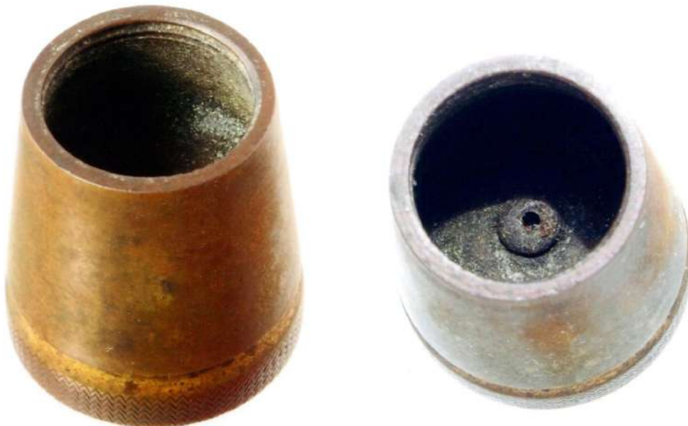
Fig. 30d: The interior of the case mouth is slightly threaded to help secure the round ball, and the base shows the end of the domed nipple.
