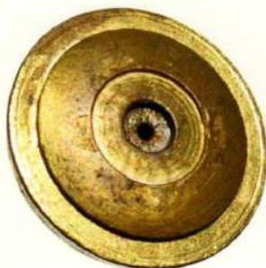
Fig. 11b: The view of the base of the turned rosette with a recess for the ignition compound and screwed-in iron disc with ignition orifice. Iron used as a more resistant metal to impact than brass. Diameter of the rosette: 22.55 mm.
