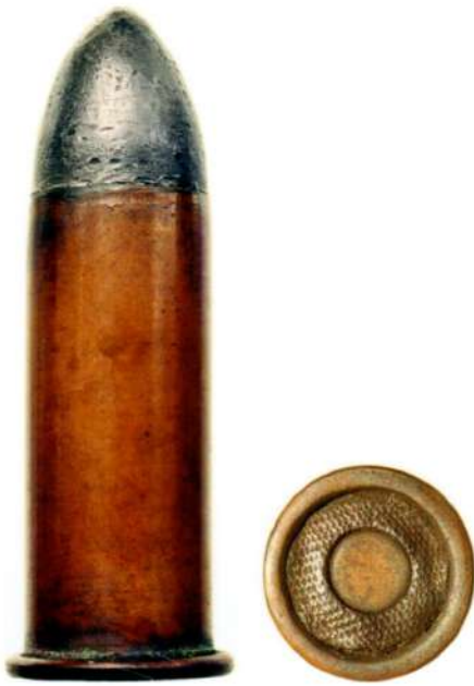
Fig. 37: .54 Morse, copper case, type I c made at Frankford Arsenal One-piece drawn copper case with a heavily rolled rim; non-ferrous flat two-pronged single wire “wishbone” anvil forming a cone with vent hole (type I c); fabricated rubber washer; simple large copper percussion cap; original smooth pointed lead bullet. Case length: 38.0 mm.
