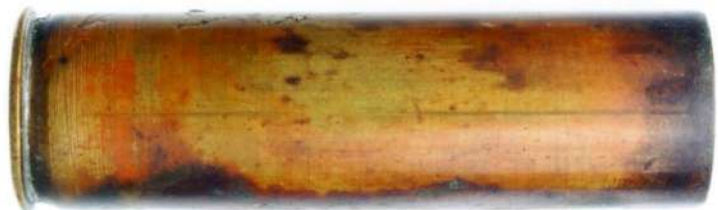
Fig. 40: .58 Confederate Morse forager shell, type I c Head of a .50 CSA Morse carbine cartridge cut off and soldered into one end of a probably cast (or drawn?) .58 inch brass tube, which has some manufacturing (casting) flaws; two-pronged sheet brass forms the cone anvil (type I c), which is identical to that one used in the .50 CSA Morse cartridge; fabric washer and copper cap; the case, which is made into a forager shell, is empty as are all the 21 shells still remaining in Bonham’s cased Morse set. Case length: 55.5 mm; interior case mouth diameter: .578 inch (14.68 mm). This cartridge has once been part of the cased three barrel Confederate brass frame Morse set presented to Milledge Luke Bonham (ca. 1864), who was Governor of South Carolina from 1862 to 1864. The cased set is on exhibition at the South Carolina State Museum, Columbia, SC.
